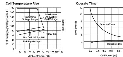
Note: Rise data is based on the max. allowable temp. for E type insulation coil (115°C).
